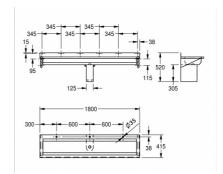
Wall mounted washtroughs with tap deck and optional rear splashbacks incorporating manual or electronic self-closing water controls, manufactured from 1.2mm thick stainless steel. 1800mm Washtrough with Tap Deck for 3 users
