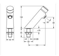
F3S Self-closing pillar tap DN 15 for sanitary facilities. Self-closing cartridge, hydraulically controlled, piston-free design, self-closing, stepless adjustment of flow duration. For connection to pre-mixed hot water or cold water. Casing, high-polished chromium-plated brass. Aerator with an integrated flow regulator 3.0 l/min.
